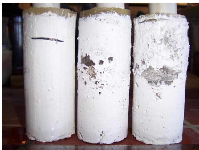
Fig. 4. Cement mortar specimens after 24 months partially immersion in 3.5 wt.% NaCl solution. From left to right: SB, Lax, Acr3.
